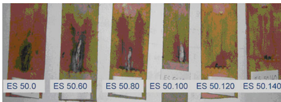
Figure 16 Test samples after tracking test IEC 587 for different ATH content. [Color figure can be viewed in the online issue, which is available at www.interscience.wiley.com .]
